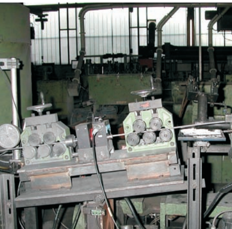
Wire inspection in drawing line
