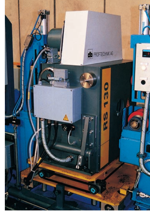
Offline testing of bright steel with RS 130 rotating system
