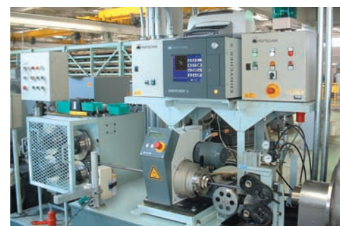
Inline inspection of spring wire
