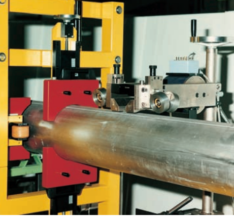
Full-body testing with multi-segment coils and weld seam inspection
